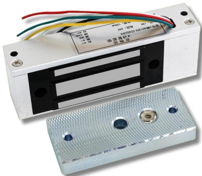
powers on to lock and powers off to unlock, providing automatic release during power failures for enhanced safety. Constructed with an aluminium alloy shell and electroplating treatment, these locks offer superior durability and resistance to wear, making them suitable for diverse applications in commercial and industrial environments.
